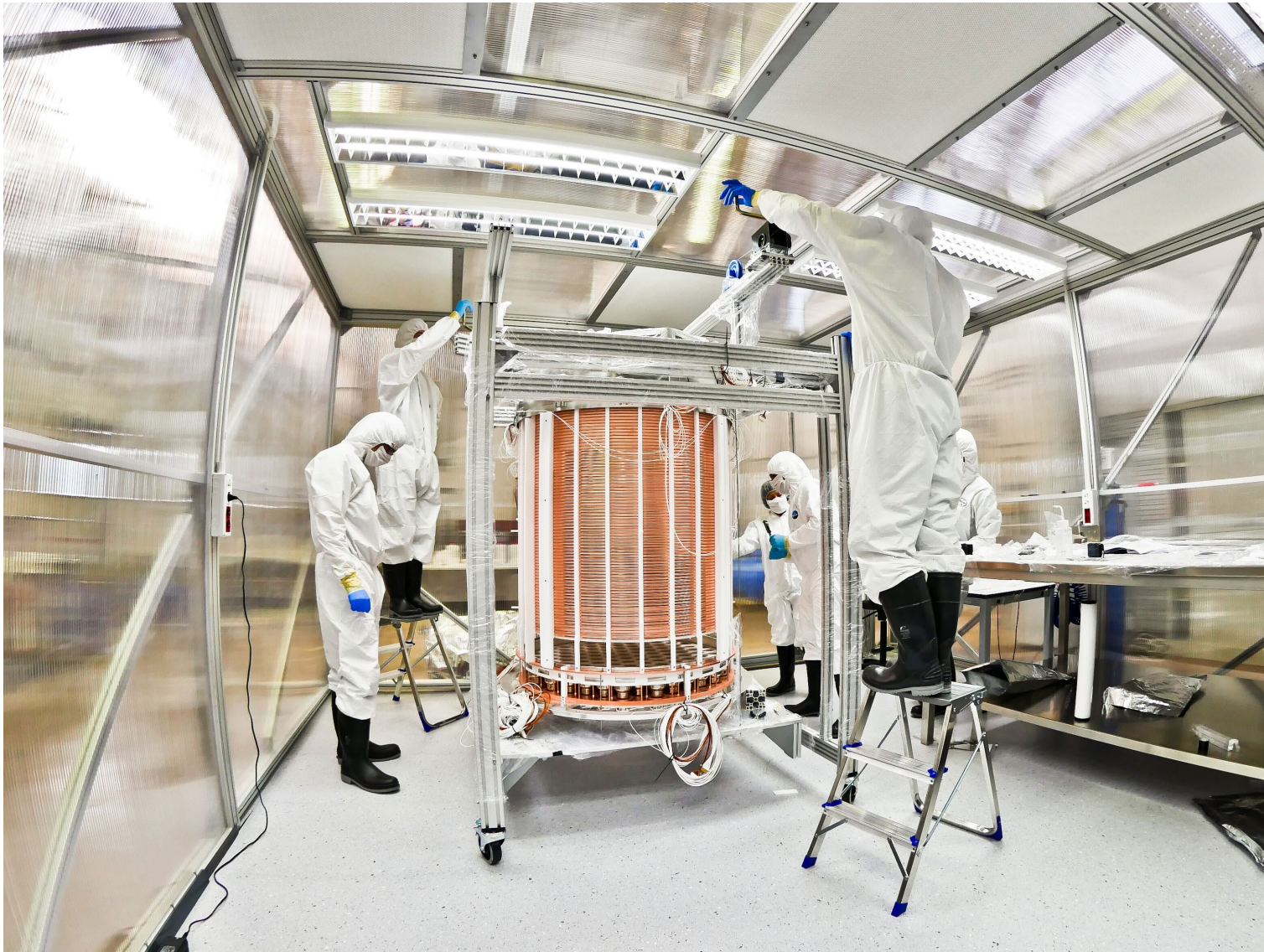
The XENON1T Time Projection Chamber TPC after assembly in a clean room: XENON Collab.
